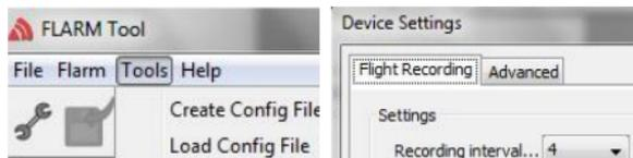
Under Flight Recording, you will find options for Recording Interval and Pilot/Airplane properties, under Advanced you can find Connection settings, Radio settings, device ID for radio communication and ICAO 24-bit address in case you have transponder.
