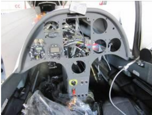
Reinstallation after panel upgrade
