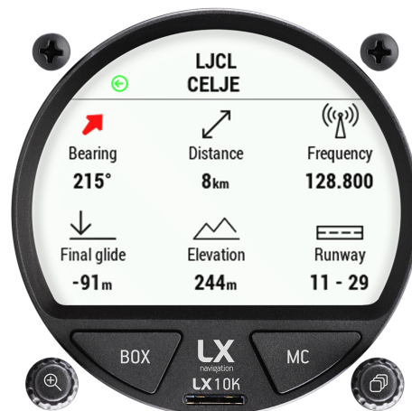
Figure 24. Airport additional info sub-page
